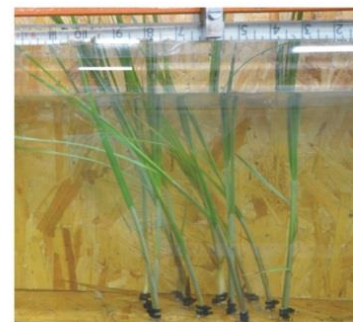
Fig. 3 Flume experiments with contrasting plant morphology (thin and long vs. thick and short). Velocity profiles were measured in front of and behind the vegetation patch.
