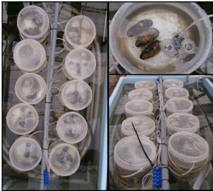
Figure 1. Experimental set-up for warming and hypoxia experiments. Image shows one temperature treatment consisting of 10 tanks receiving continuous supply of fresh seawater (at experimental temperature). Half of tanks received hypoxic water for final week of 28-day exposure.
